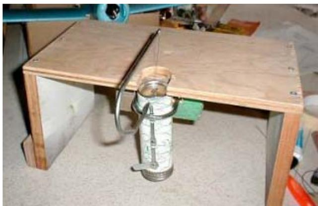
Here's a quick, cheap and a little bit dirty hot wire cutting table based on the portable Wonder Cutter tool available from Foamfly.com for \$13.50. The tool works with two "D"cells and the wire draws about 1.25A so a pair 1250ma. cells should last more than an hour. Scrap wood was used and a 2-1/4" U-bolt form my junk box.
