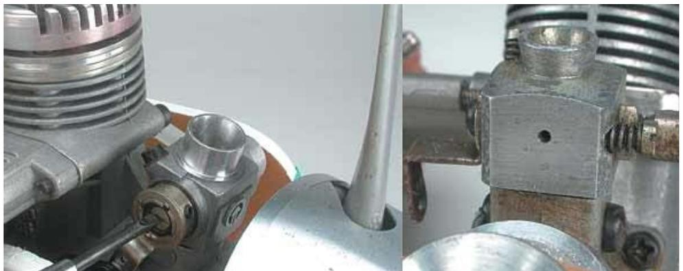
**A reliable idle is very important, especially during landings. A carburetor can have either a low-end needle-valve adjustment (left) or an air-bleed hole in the front of the carb housing (right). Adjust the high-end needle valve be-**
