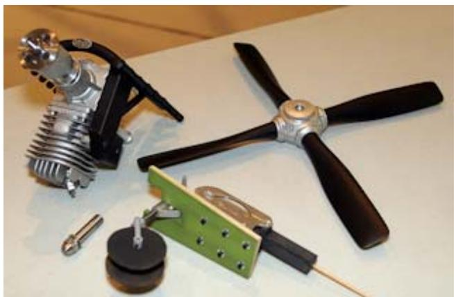
At our last meeting Simon Nadler bought along a DL50 sporting a Keleo Creations scale functional exhaust, a Sierra Prop extension and NRG Soloprop unit featuring a ground-adjustable pitch 18" propeller.
